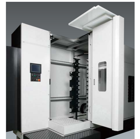
Open ceiling magazine door
