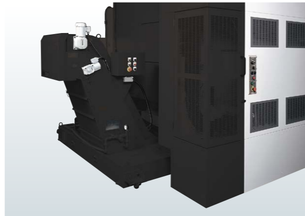
Lift-up chip conveyor (Optional)
