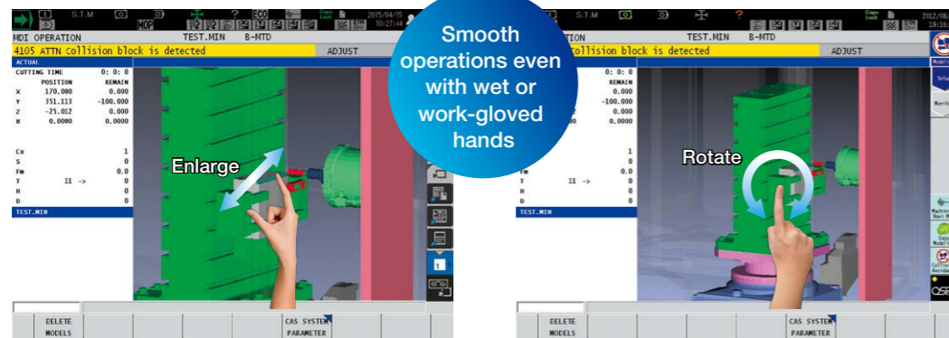
Note: 15-in. operation panel screen shots. Collision Avoidance System (Optional) shown above.
