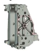
Diagonal rib configuration of columns
