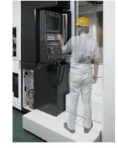
Good access to machine interior with wide, 2-step platform
