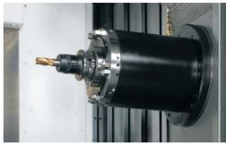
Long service life oil-air lubrication (all spindles)
