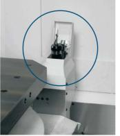
Probe type sensor Detection increment: 1 µm Auto-measure aligning air blower quipped
