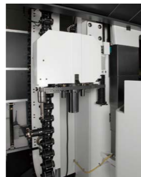
Next tool readied during machining operation
