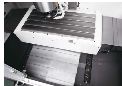
In-machine chip discharge: Coil MILLAC 468VII
